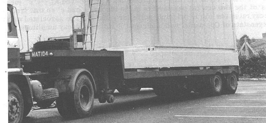
Figure 19. Loading one of the standard containers used to transport apparatus to CERN. The containers were specially fitted before leaving the Rutherford Laboratory to enable them to be quickly interconnected at CERN to make the control room for experiment 14.
