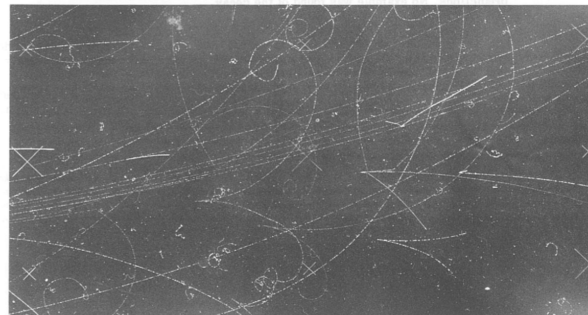
Figure 26. An example of a \Xi^0 interaction photographed in the UCL - RHEL heavy liquid chamber. The \Xi^0 is produced in the reaction K^- + p \rightarrow \Xi^0 + K^0 , K^0 \rightarrow \pi^+ \pi^- . The \Xi^0 charge exchanges in the reaction \Xi^0 + p \rightarrow \Xi^- + \pi^+ + p , \Xi^- \rightarrow \Lambda^0 + \pi^- , \Lambda^0 \rightarrow p + \pi^- . The \pi^+ from the \Xi^0 interaction scatters on a proton.
