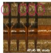
White corrosion residue visible with low-angle lighting. Traces of chlorine detected on ENIG surface
