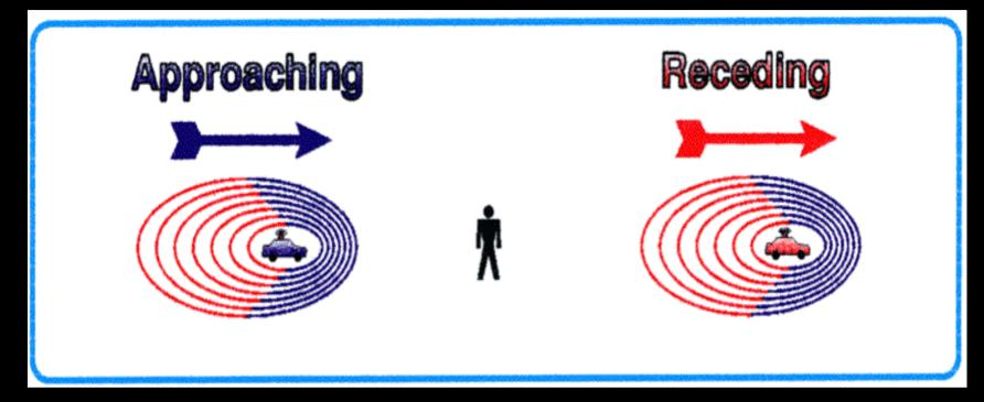
Frequency increasing Wavelength decreasing Wave crests get closer together Colour gets BLUER = BLUESHIFT Frequency decreasing Wavelength increasing Wave crests get further apart Colour gets REDDER = REDSHIFT
