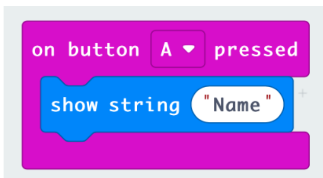
Figure 1 Model code for the introduction exercise. When programmed this will show the pupil's name when they press the A button.
