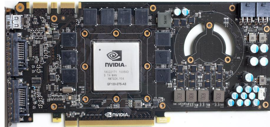
NVIDIA GTX460 card (heat-sink and cooler removed)
