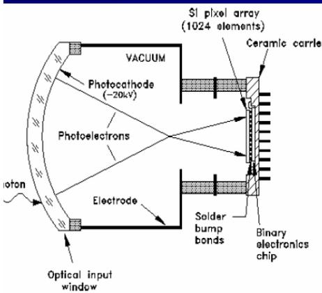
Readout: Hybrid PhotoDiodes HPD
