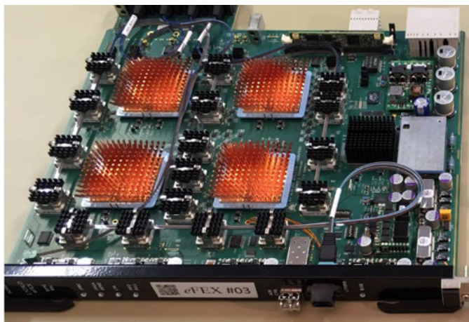
Figure 3.2: eFEX prototype, showing copper heatsinks on top of the large FPGAs, and sockets for the on-board optical connections.
