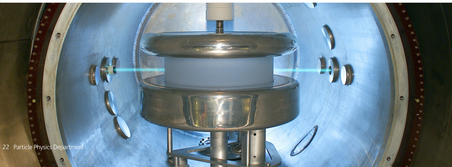
Figure 4.2: The completed room-temperature nEDM experiment: ultra-cold neutrons are stored in a quartz cylinder in an electric and magnetic field. A Hg co-magnetometer probes the storage volume for magnetic field fluctuations to a precision of 1 nGauss that enabled the most precise nEDM measurement to date to be made.
