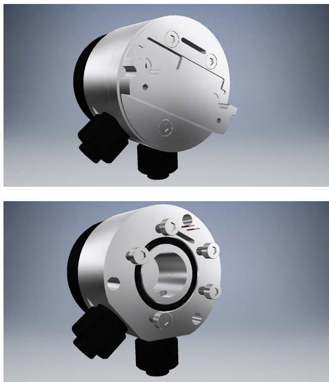
Figure 10.2 : CAD models of the modified CCD mount and heatsink used in the Global Jet Watch telescope cameras.
